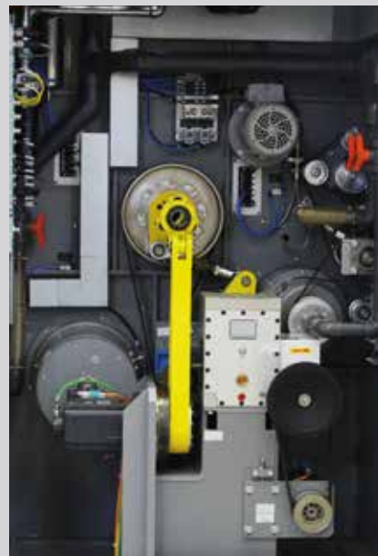
Compact servo drive concept with separate servo drives for stroke and transport movement and good accessibility for maintenance
