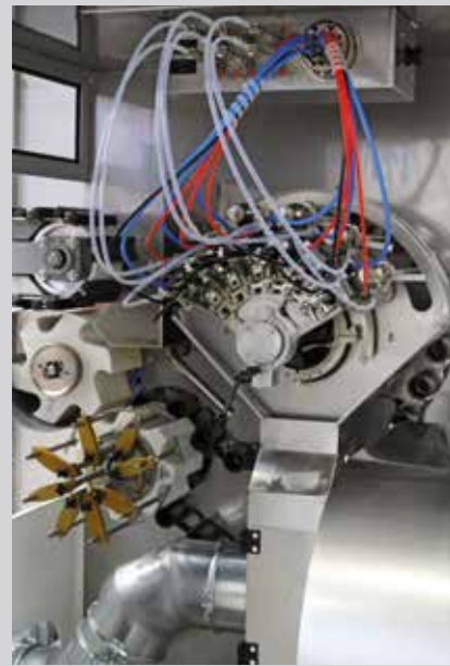
6/4 spray gun holders with quick-change infeed system
