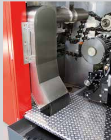
Automatic part ejection during production process (single or group pre-set)
