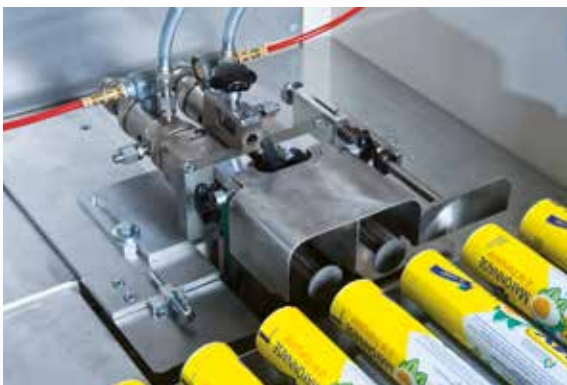
Latexing with 2 high-end centrifugal guns S-540 on format-independent conveyor belt
