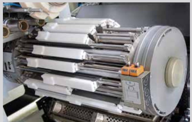
Proven transfer concept by combined transfer drum to the internal drier
