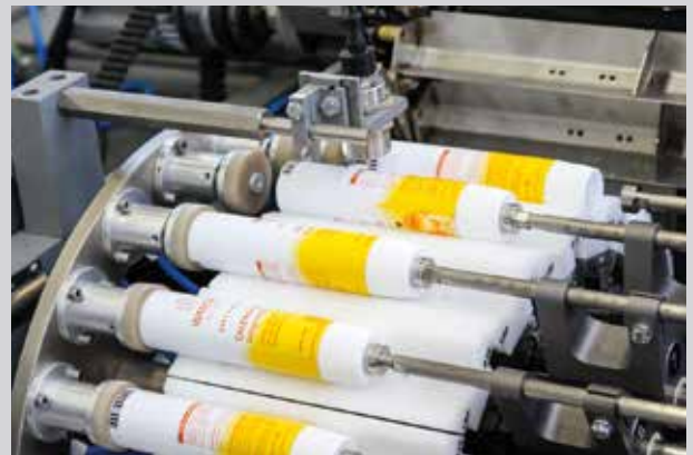
20 testing heads test up to 200 aluminum tubes per minute for leaks with diameters starting from 0.04 mm
