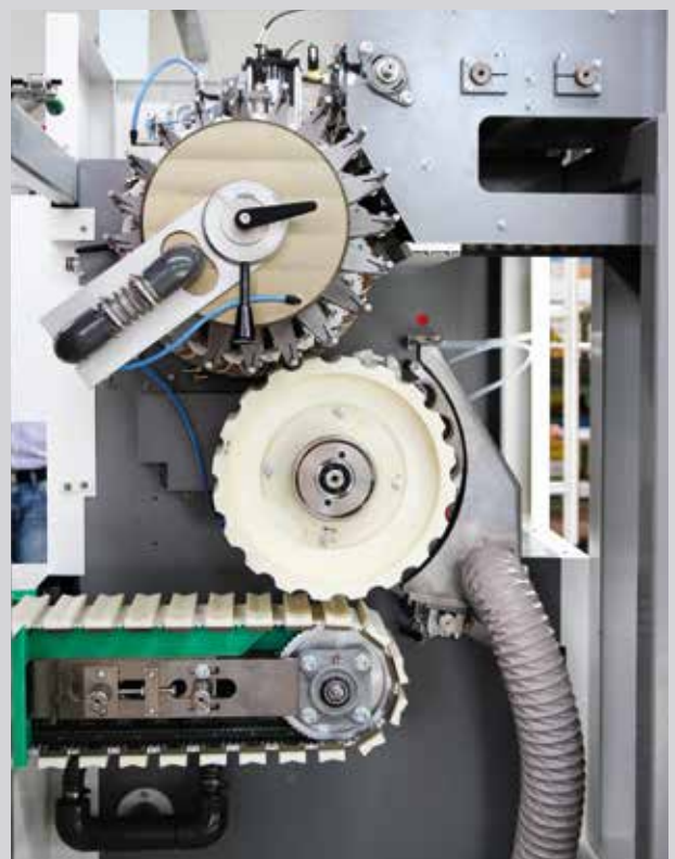
Drum concept for precise positioning of the aluminum tubes
