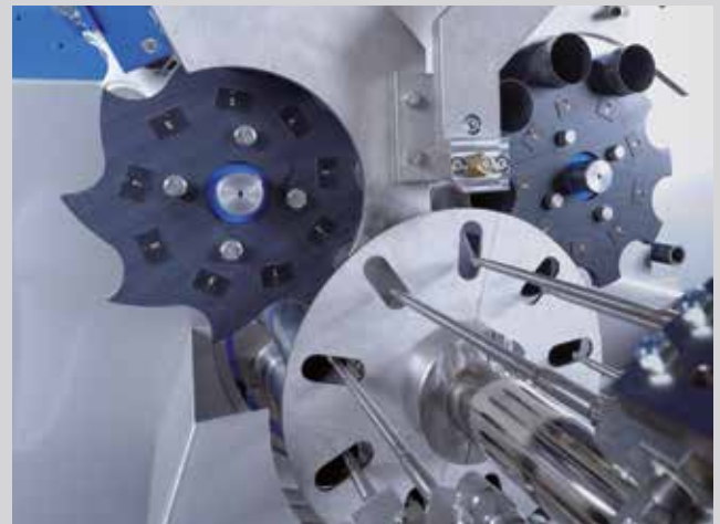
Can transfer by infeed starwheel, central vacuum disc and outfeed starwheel
