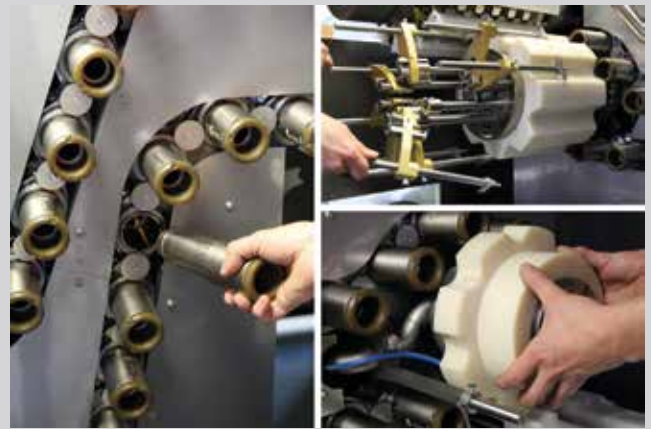
Quick-change system for size parts
