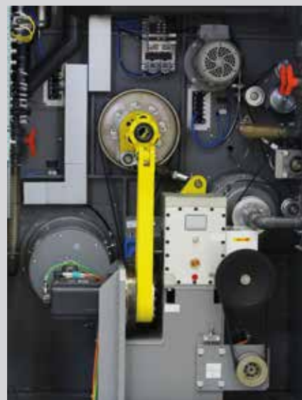
Compact servo drive concept with separate servo drives for stroke and transport movement and good accessibility for maintenance
