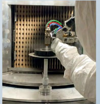
The coating robot is equipped with two Sprimag spray guns, thus different requirements regarding the coating layer can be met
