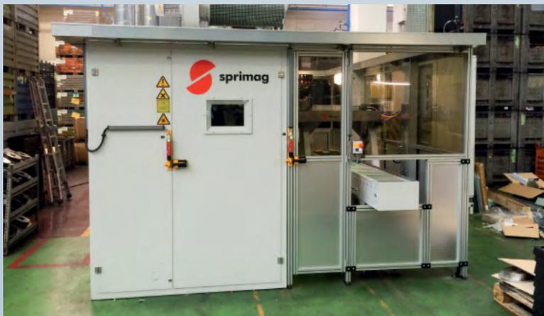
UV-coating machines are particularly compact, as no exhaust air section and cooling zone is required
