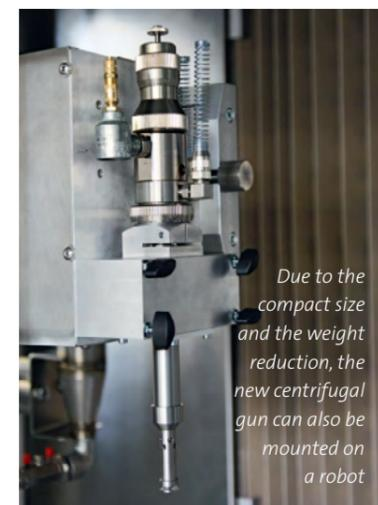
Due to the compact size and the weight reduction, the new centrifugal gun can also be mounted on a robot
