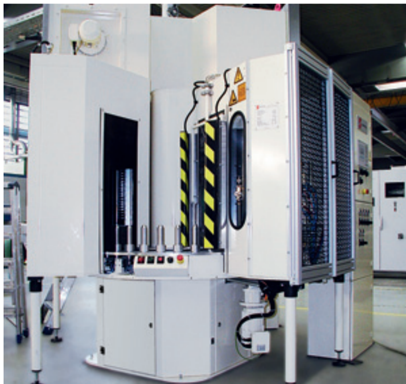
Round Table Coating Machine for rubber to metal bonding parts alternatively also available with coating robot
