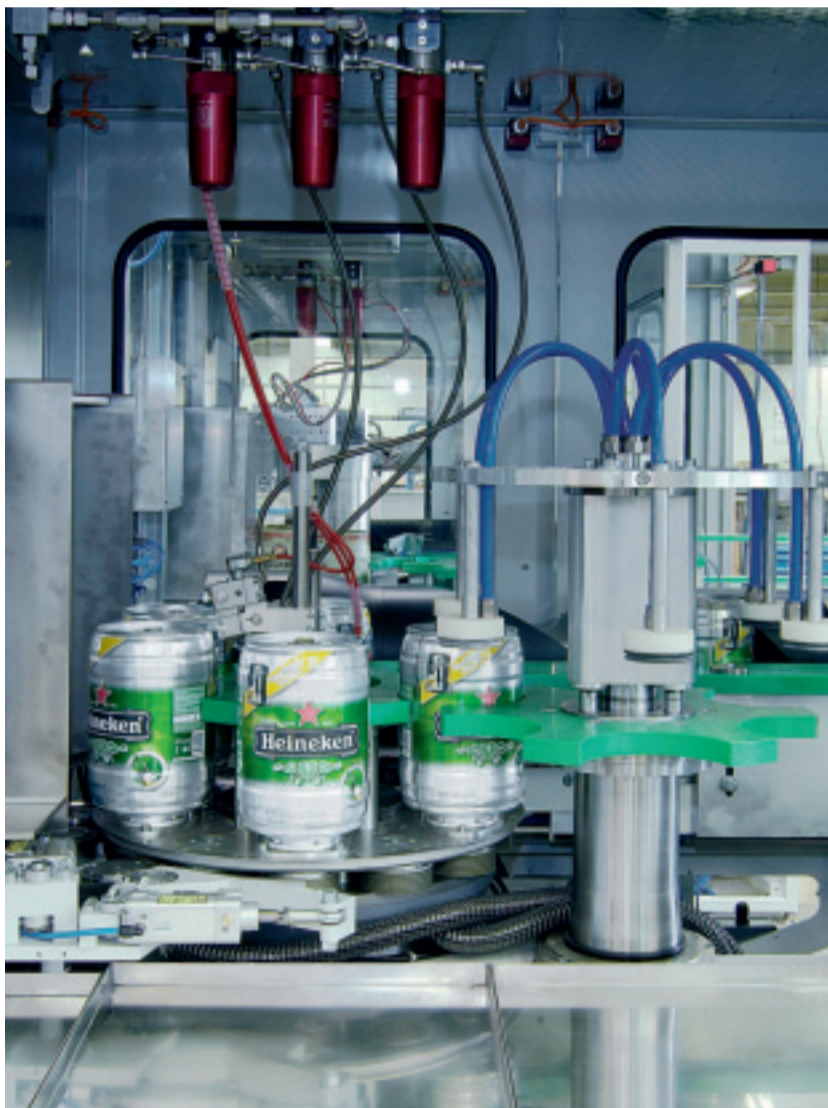
By inner coating of party kegs Sprimag ensures good taste
