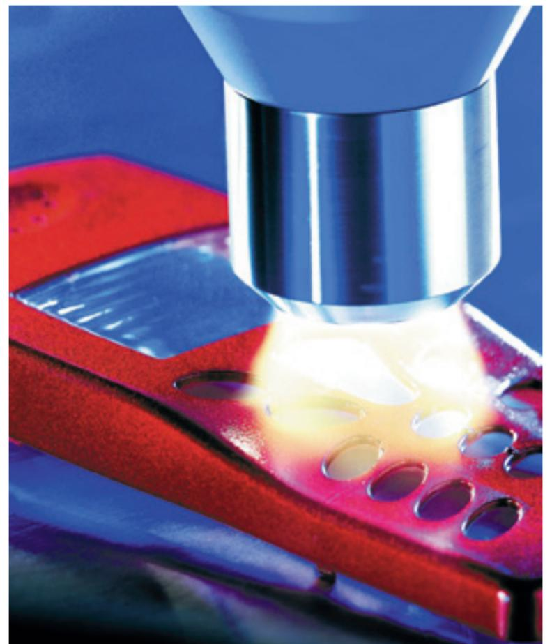
Plasma technology is increasingly being used as a pre-treatment process in complete coating systems
